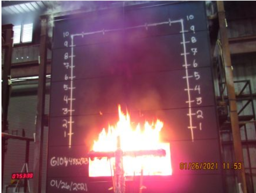
Photo No. 25 Flame height at 2 ft above window
