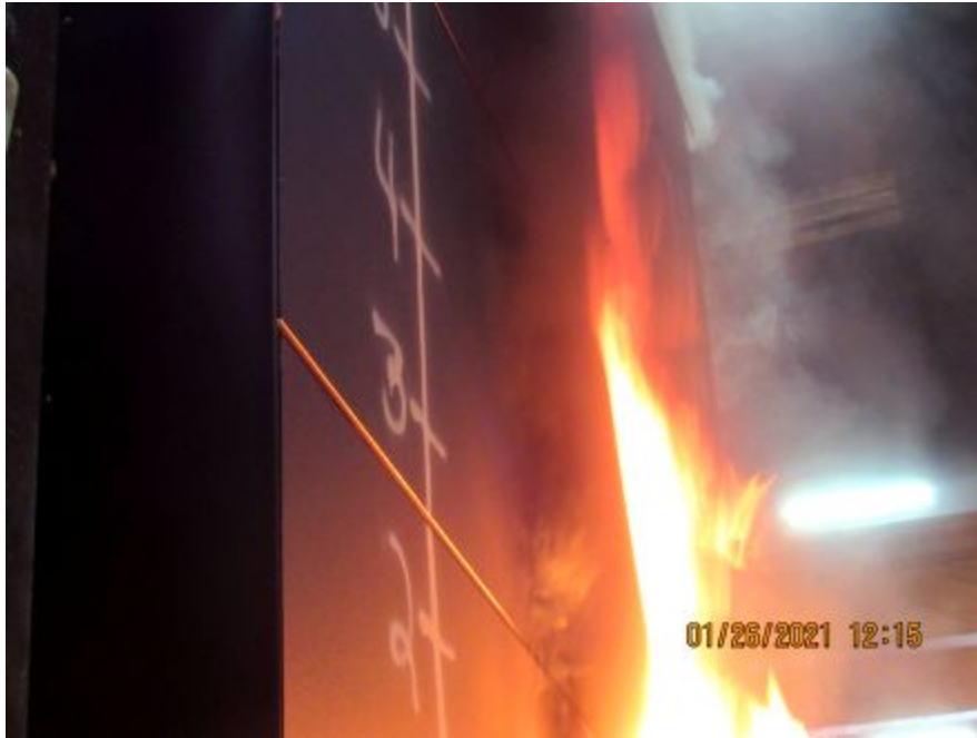
Photo No. 29 Second row panels opening up
