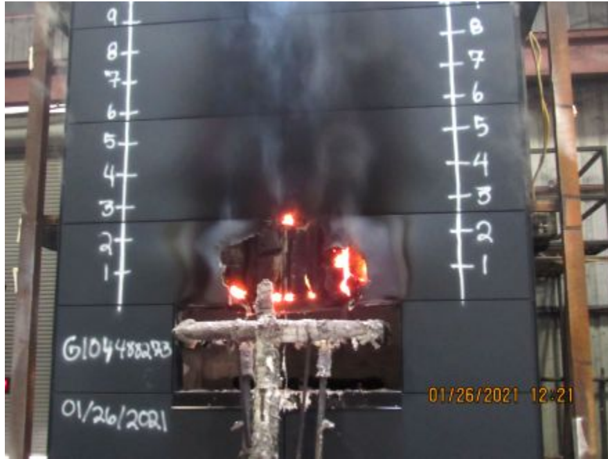
Photo No. 31 Residual flaming post-test
