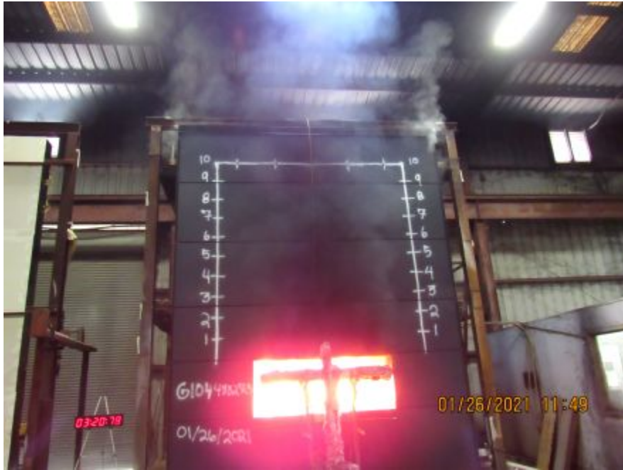
Photo No. 23 Smoking from top of wall
