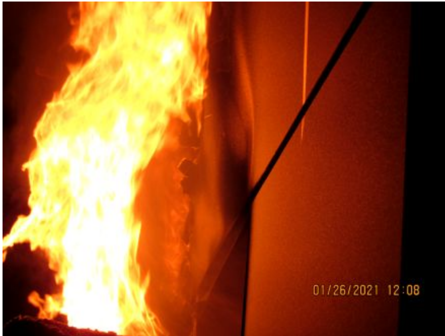
Photo No. 28 Panels opening up
