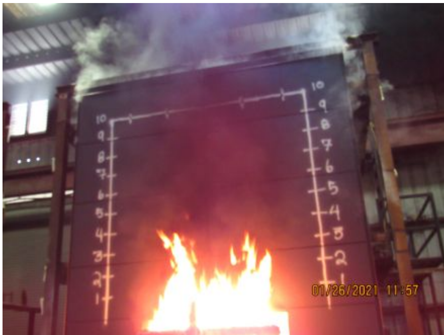
Photo No. 26 Flame tips increasing
